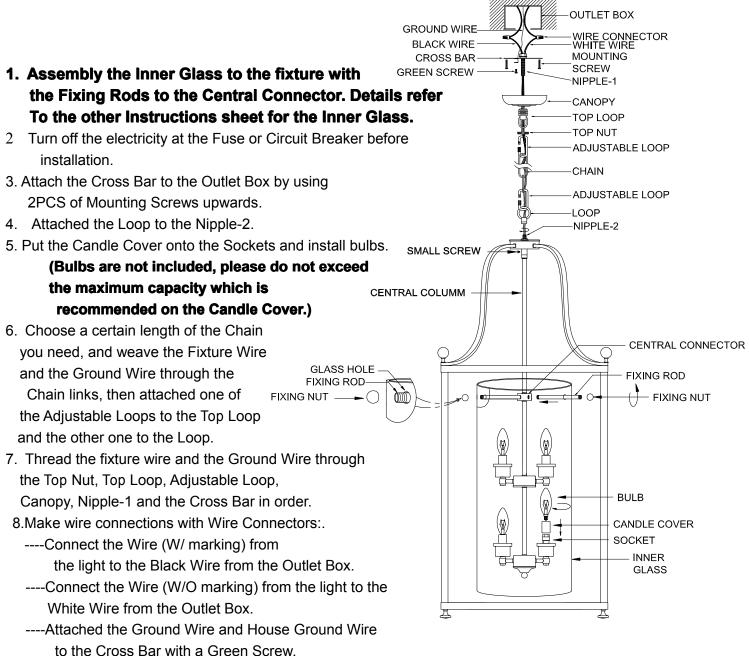
Carefully tuck wires back into the Outlet Box.
