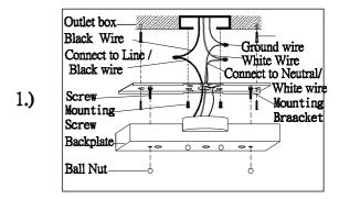
Step.1: Remove mounting bracket from fixture and install to electrical box. Wire fixture to wires in outlet box. Copper wire is for Ground. On wire side
